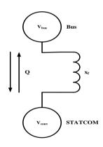
Figure 5. Principles of STATCOM operation
