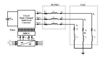
Figure 2. MPCC based FLDCMLC control
