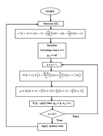
Figure 3. Flow chart of MPCC for FLDCMLC
