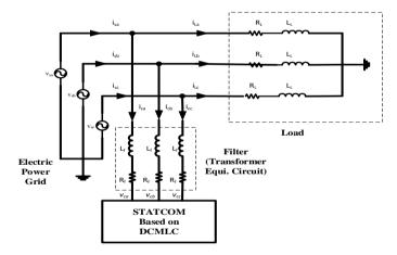
Figure 4. Basic connection of STATCOM
