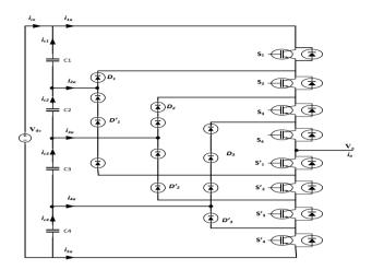
Figure 1. Structure of Five Level Diode Clamped Multi-Level Converter FLDCMLC
