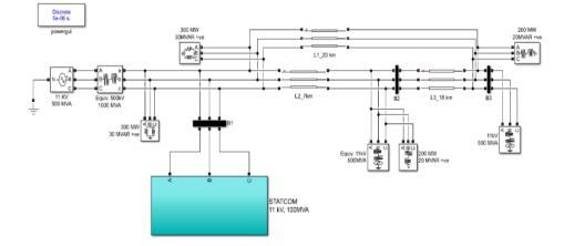
Figure 6. STATCOM based on FLDCMC
