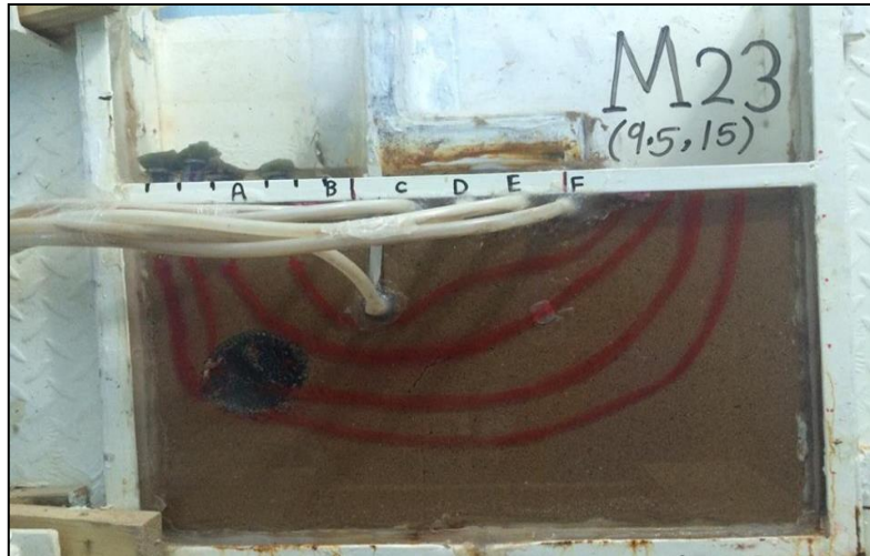
Fig. 3. Typical flow lines pattern for model \frac{b}{B} = 0 with cavity \frac{y_c}{T} = 0.5 and \frac{x_c}{B} = -0.74 .
