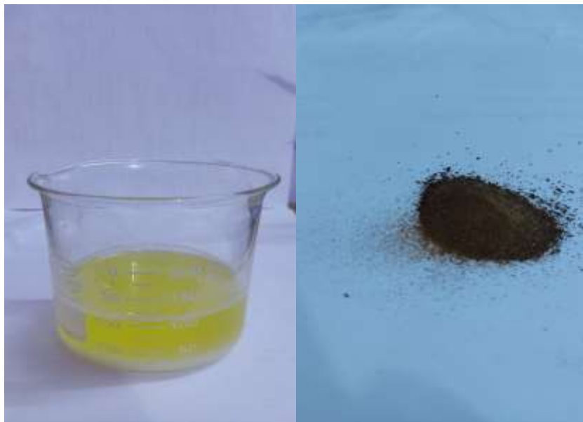
FIGURE 1. (A) pale yellow ZnONPs after mixing with BC. (B) ZnO nano powder dried in oven at 60 °C.
