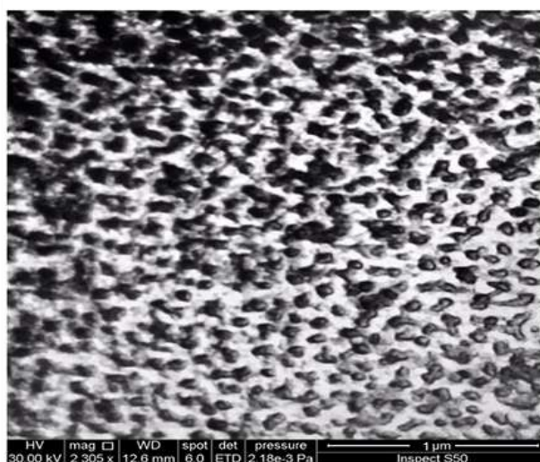
Figure 3: Electron microscopic image(1 \mu m) of selenium loaded Ribes nigrum nanoparticles 1:2 ratio at pH 9
