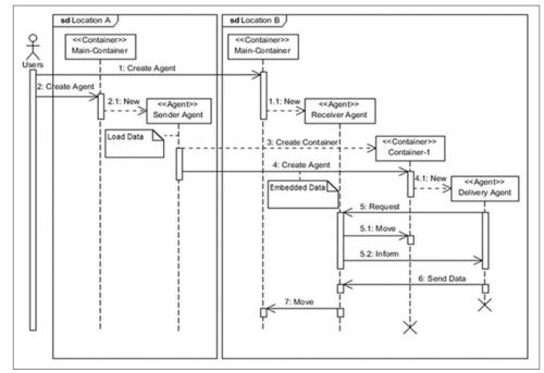
Figure 4: AUML sequence diagram of proposed communication method for multi-agent system
