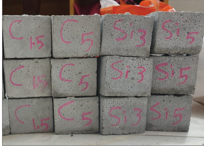
FIGURE 3. Specimens of compressive strength test
