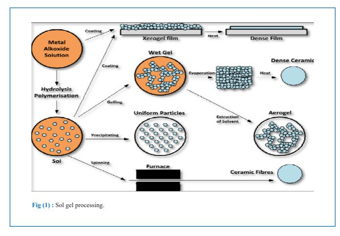
The processes are shown in Fig.1. are by no means restrictive or complete. These steps may be extended, modified, or completely removed except for solvation and gelation, depending upon the specific application [12]. The stages of hydrolysis and condensation reactions are constant in the production of sol-gel-derived bioactive materials. This section describes the routes of soil gel synthesis for biomedical ceramic and glass networks that are most frequently used [11].2.1 Enhancing in sol-gel:
