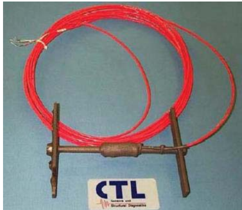
FIGURE 2. CTL asphalt strain gauges
