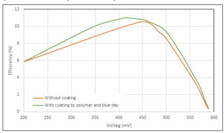
Figure 7 The relationship between efficiency and voltage with and without coating.
