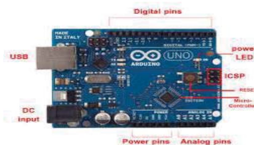
FIGURE 3. Inside connection of Arduino [13].
