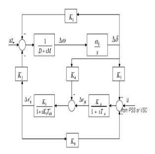
Figure 4: The linearized model of power system
