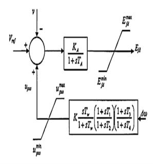
Figure 2:Block diagram of PSS and excitation System
