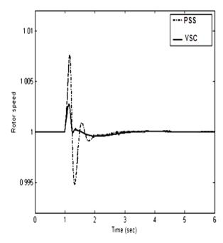
Figure 9: Response of generator rotor speed at nominal loading
