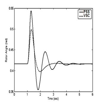
Figure 10: Response of generator rotor angle at light loading
