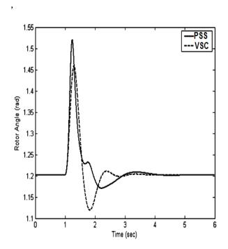
Fig 8: Response of generator rotor angle at nominal loading
