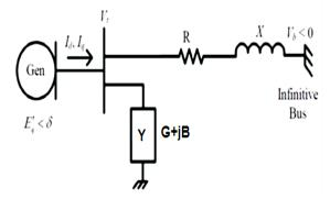
Figure 1: single machine infinite bus system
