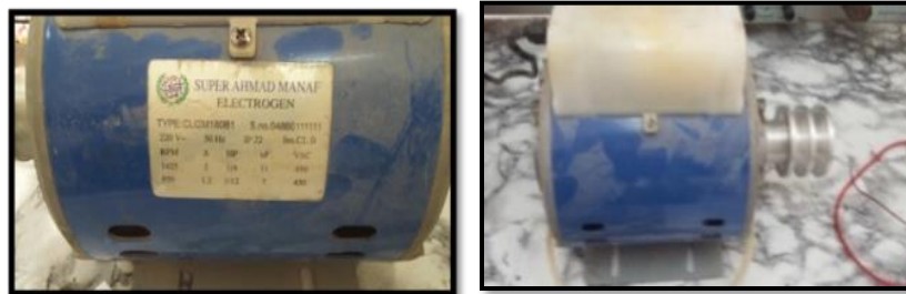
Figure 10: Single Phase Induction Motor is a Type of Squirrel Cage
