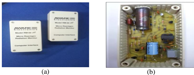
Figure 2: the appearance of RM-60 radiation monitoring system; (a) outside, and (b) inside where a LND712 Geiger-Muller (GM) tube
