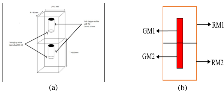
Figure 8: The schematic diagram of a cosmic ray muon telescope; (a) front view, and (b) side view
