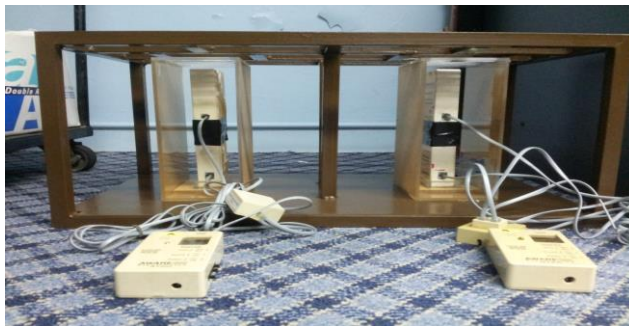
Figure 10: Two sets of MT experiment set up (2 metals simultaneous Cu and Al) inside the building)
