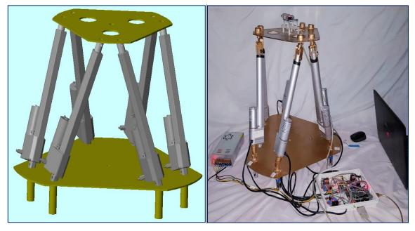
Fig (2): The model of Gough-Stewart manipulator.
