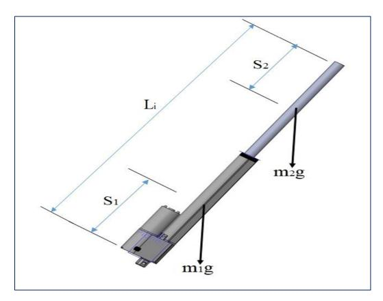
Fig (4): Two parts of i linkages.
