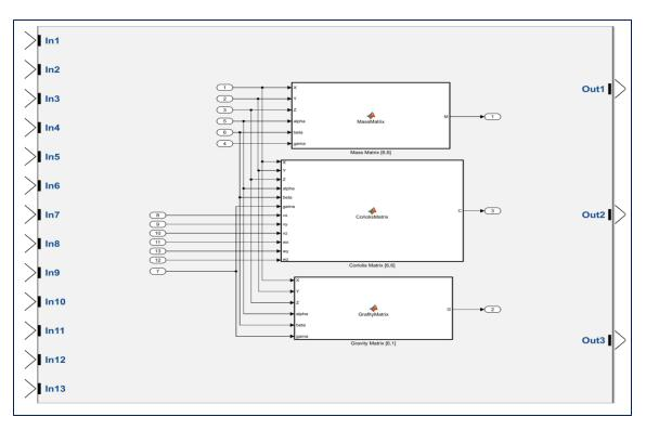
Fig (9): Mass, Coriolis, and Gravity matrices in Simulink.
