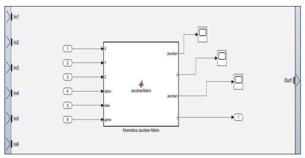
Fig (8): Inverse kinematics and jacobian blocks.
