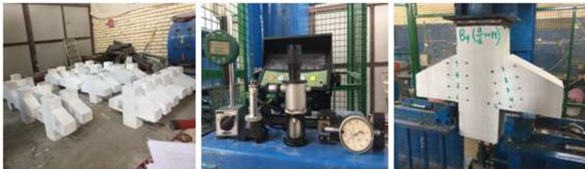
Figure (5) Represent of Corbels Specimens and Testing Machine
