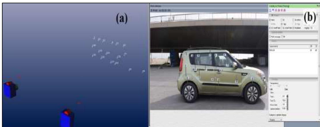
Figure 4 3D target point representation using PMS ; (a) 3D point model, (b) The residuals in target points
