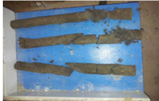
Figure 7. Three columns group after extraction from the soil
