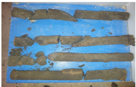
Figure 9. Three columns group after extraction from the soil .
