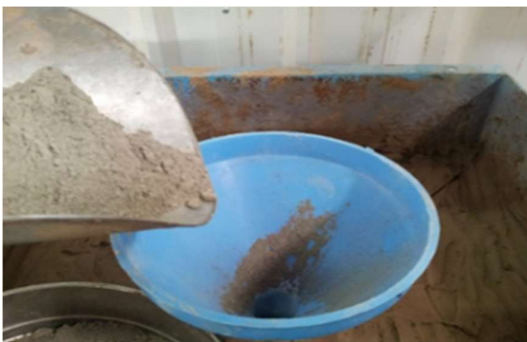
Figure 5. Fill the hole with cement or lime powder
