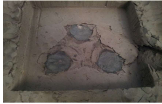
Figure 6. Three columns group after testing
