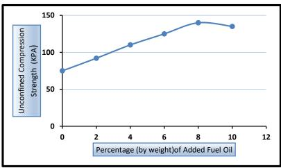
Fig. 4. The Effect of Fuel Oil on Unconfined Compression Strength
