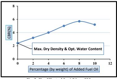
Fig. 3. The Effect of Fuel Oil on CBR
