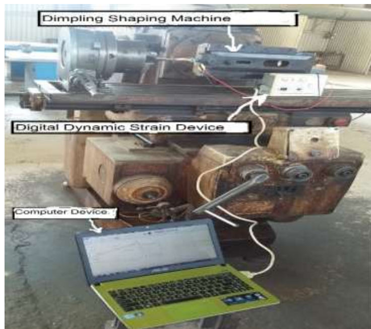
Figure 14. Practical attaching of experimental parts for strain readings
