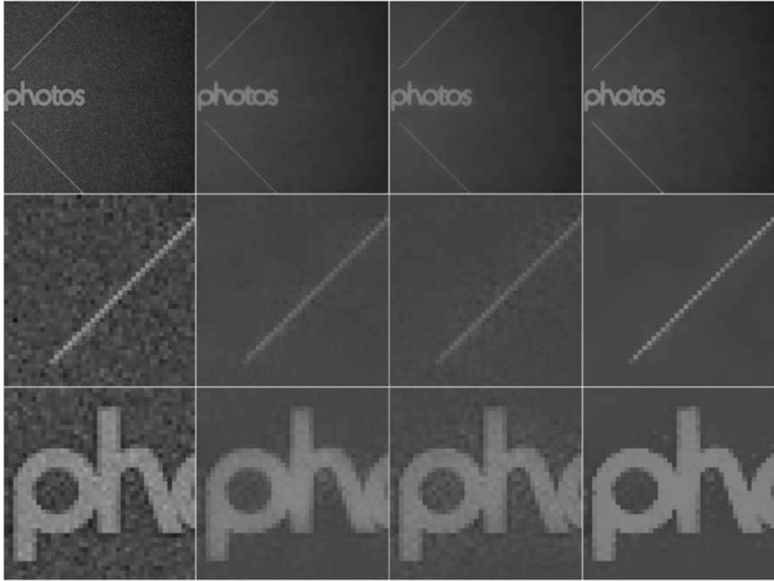
Fig. 10 Edge-aware image filtering results. All filters are tuned to produce similar PSNR. Top row, from left to right: input, BMA mode 3 ( r = 3 , \sigma_s = 255 \times 10^{-6} , PSNR = 30.41), GIF ( \epsilon = 0.0105 , \omega = 11 , PSNR = 30.43), our method ( \sigma_s = 4.5 , \sigma_r = 0.1 , 5 iterations, PSNR = 30.40). Middle and bottom row are close-ups of corresponding images in the top row
