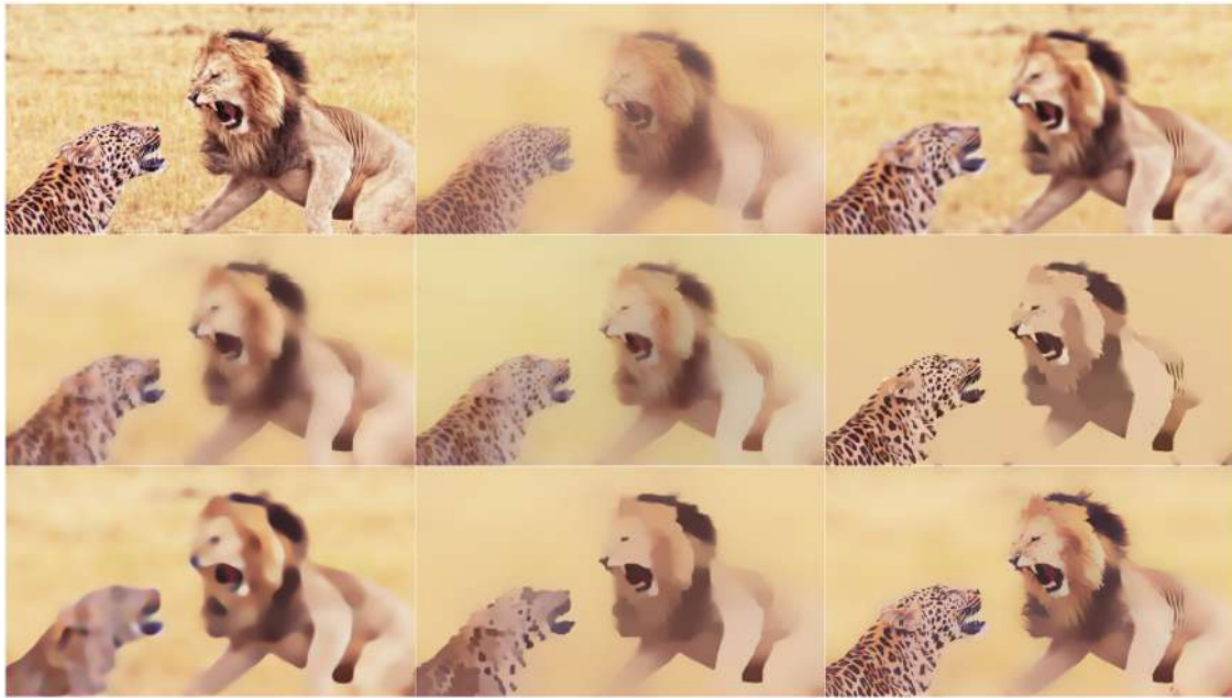
Fig. 9 Background smoothing results. All filters are tuned for their best performance in terms of background smoothing. From left to right and top to bottom: input, BMA ( r = 25 , \sigma_s = 0.00005 ), BM3D ( \sigma_s = 250 ), DMT ( \sigma_s = 20.5 , \sigma_r = 1.5 , 5 iterations), WLS ( \lambda = 2.5 , \alpha = 1.5 ), L0 ( \sigma_s = 0.075 ), RGF ( \sigma_s = 9.5 , \sigma_r = 0.05 , 5 iterations), RTV ( \lambda = 0.05 , \sigma = 3 , 3 iterations), our method ( \sigma_s = 6.5 , \sigma_r = 0.1 , 7 iterations)
