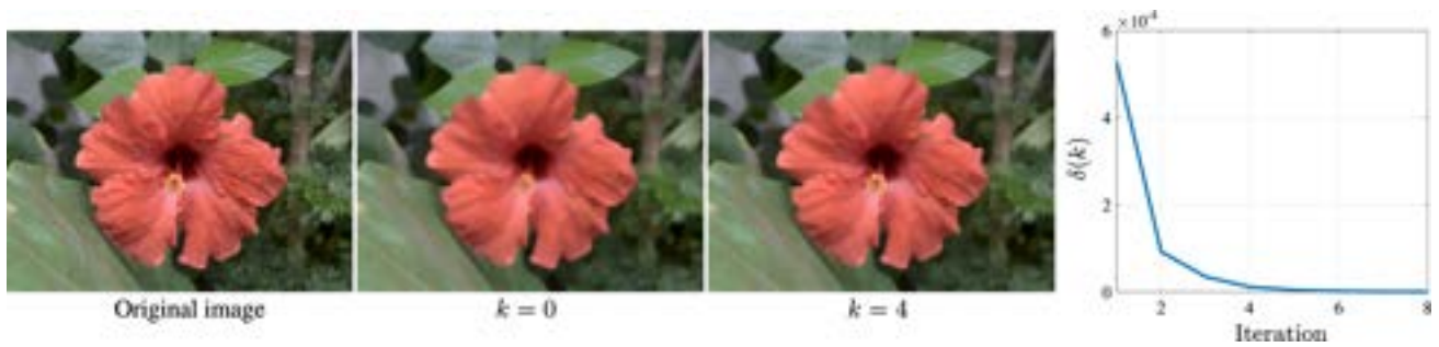
Fig. 1 The convergence of the proposed algorithm as iteration increases from the initial smooth image ( S ) ( k = 0 ) to the image at iteration ( k = 4 ). The mean squared difference \delta(k) is also shown
