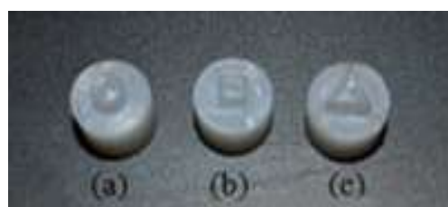
Figure 2. Types of indenters employed:(a) circle; (b) square; (c) triangle.
