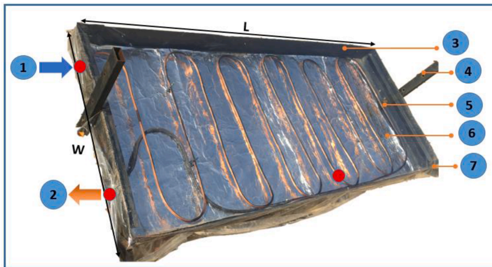
Fig. 1. A flat plate solar collector experimental design: (1) inlet from tank 1; (2) outlet to tank 2; (3) collector enclosure; (4) angle guide rod; (5) serpentine absorber tube; (6) fiberglass insulation; (7) plastic sheet cover.
