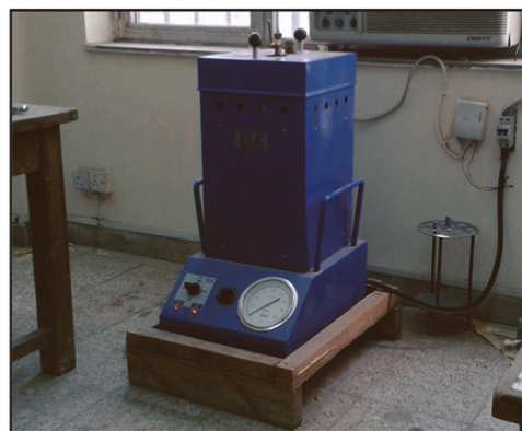
Plate 1. ELE apparatus for autoclave curing.
