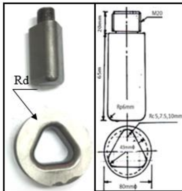
Fig. 3. A triangle tool of deep drawing.
