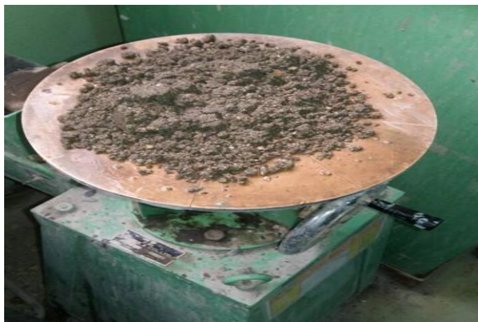
Figure 7: Flow shape of mortar mixture with 3.5% non-incinerated waste paper ash.
