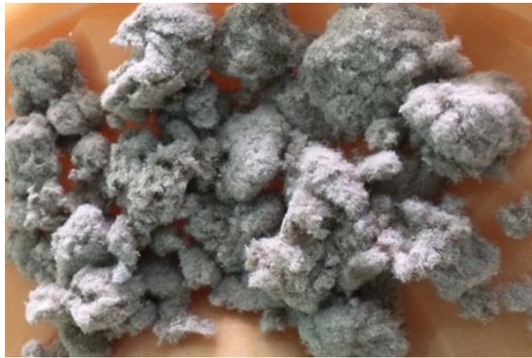
Figure 1: Waste paper before incineration (fibres).
