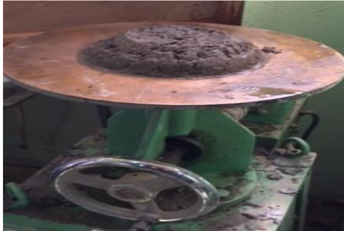
Figure 6: Flow shape of mortar mixture with 10% incinerated waste paper ash.
