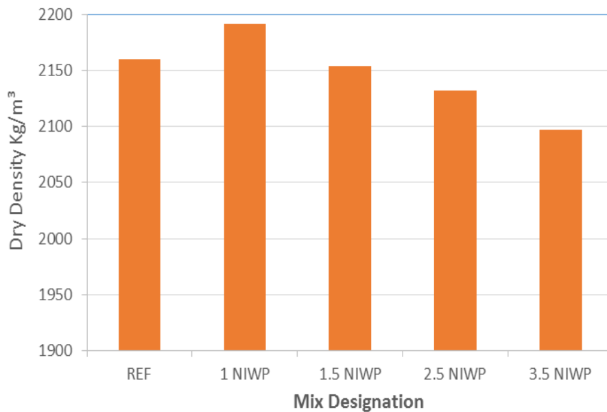
Figure 14: Dry density results of non- incinerated waste paper mixtures at 28 days.
