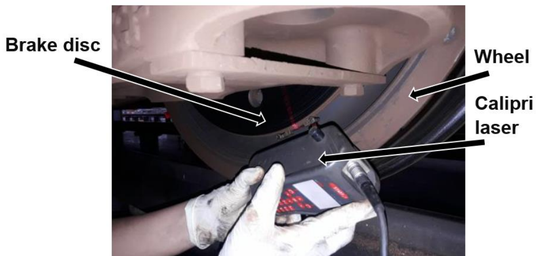
Figure 4: Measurement of brake disc wear profile using Calipri laser.
