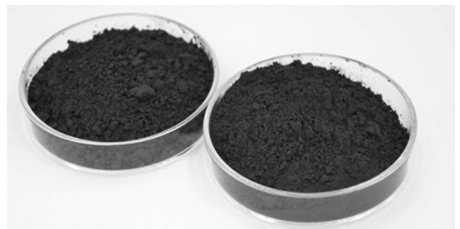
Fig.4. Carbon resulting from the activation of date seeds.
