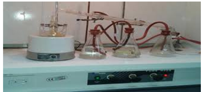
Fig.3. Experimental device for preparing activated carbon.
