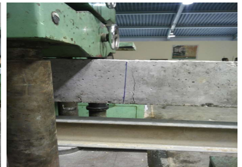
Plate 3. Beam flexural cracks.
