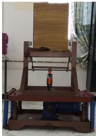
Figure 14. Duplicated picture for whole assembly of driver's seat test rig.
