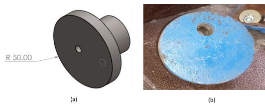
Figure 3 a. Sketch of eccentric cam in SOLIDWORKS program b. Photograph for the eccentric cam
