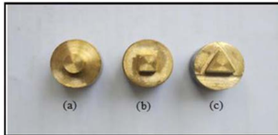
Figure 2. The utilized tips of indenter: (a) Circle; (b) Square; (c) Triangle.
