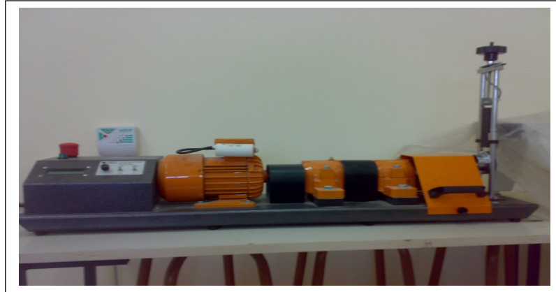
Fig. 1 Fatigue Tester by bending at Technical Institute, AL-Musaib, mechanic department.
