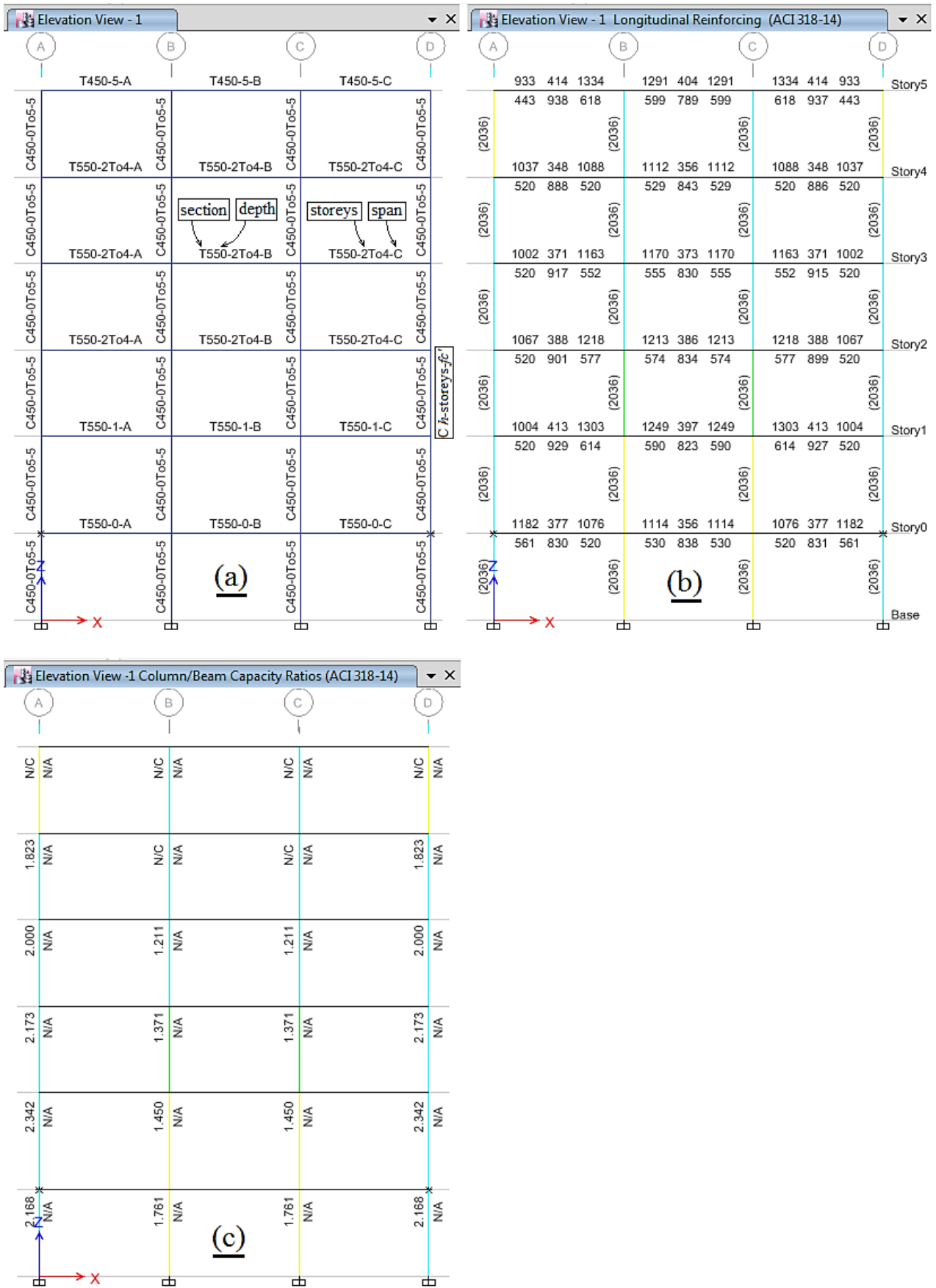
Figure 7. Archetype model frame of 6 m bay width and five stories height; a) Members sections, b) longitudinal reinforcing, c) column / beam capacity Ratios
