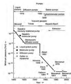
Fig. 8. Pressures of vacuum, achieved in the period from 1900 to 2000 [23].
