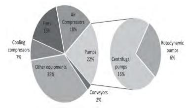
Fig. 3. Energy consumption for different applications [16].
