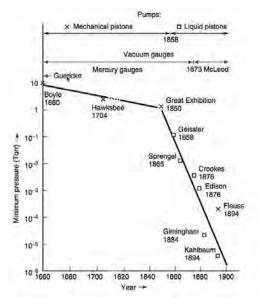
Fig. 7. Pressures of vacuum, achieved in the period from 1660 to 1900.
