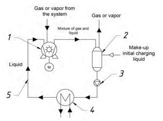
Fig. 2. A schematic diagram of major system components of LRVPs: 1 – LRVP; 2 – separator vessel; 3 – liquid circulating pump; 4 – water cooler; 5 – pipelines.
