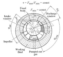
Fig. 13. The basic traditional design of LRVP [45].
