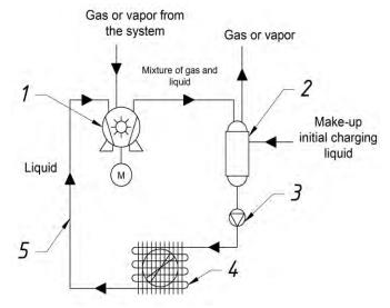
Fig. 10. LRVPs unit with air cooler of circulation working liquid: 1 – LRVP; 2 – Separator vessel; 3 – Liquid circulating pump; 4 – Air cooler; 5 – Pipelines.
