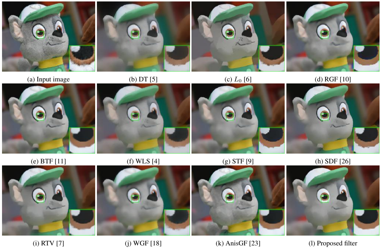
FIGURE 7: A comparison of edge-preserving image smoothing with a group of state-of-the-art algorithms. (a) Original image, (b) DT ( \sigma_s = 30, \sigma_r = 0.7, N_{iter} = 5 ), (c) L_0 ( \lambda = 0.02, \kappa = 2, N_{iter} = 1 ), (d) RGF ( \sigma_s = 5, \sigma_r = 0.1, N_{iter} = 20 ), (e) BTF ( k = 5, N_{iter} = 5 ), (f) WLS, ( \lambda = 1, \alpha = 1.2 ), (g) STF ( \sigma_s = 3, \sigma_r = 0.08, \sigma = 0.01, N_{iter} = 4 ), (h) SDF ( \sigma_g = 50, \sigma_u = 400, \lambda = 30, nei = 1 ), (i) RTV ( \sigma = 3, \lambda = 0.015, \epsilon = 0.02, N_{iter} = 4 ) (j) WGF ( \sigma = 1, \epsilon = 0.01, N_{iter} = 10 ) (k) AnisGF ( \sigma = 1.5, \epsilon = 1 ) (l) Proposed rolling GVWA Type-II filter ( \sigma_s = 1.5, s = 0.75, N_{iter} = 20 ).
