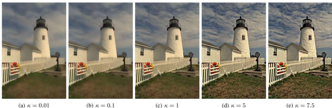
FIGURE 4. Effect of varying \kappa for settings r = 11 , \epsilon = 0.01 , scale = 1 . (a) and (b) Smoothing ( 0 < \kappa < 1 ). (c) Original image ( \kappa = 1 , no filtering). (d) and (e) Sharpening ( \kappa > 1 ).
