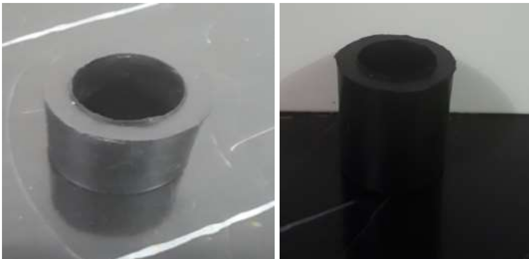
Figure 13 Show the rubber bushing product Manufactured
