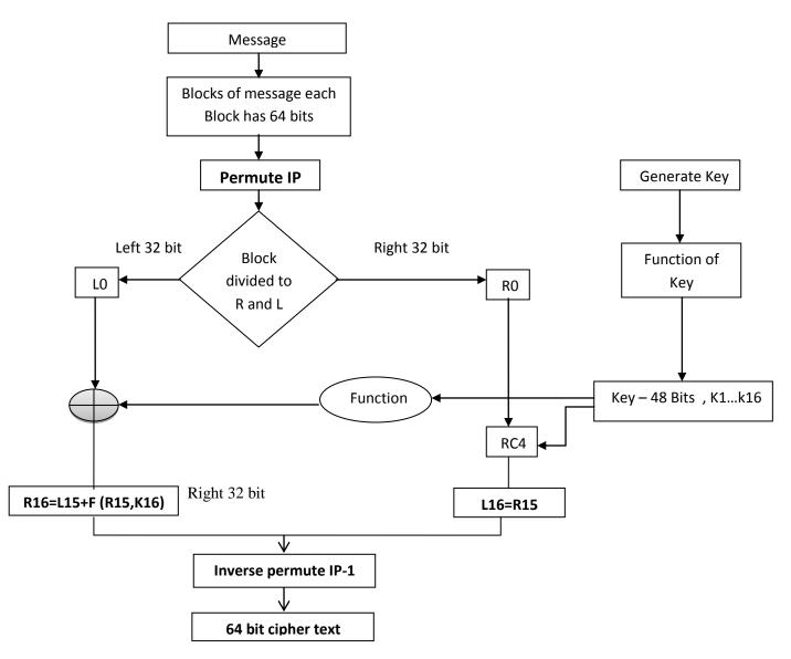
Figure 1: Flowchart to Explain Combining (DES & RC4)
