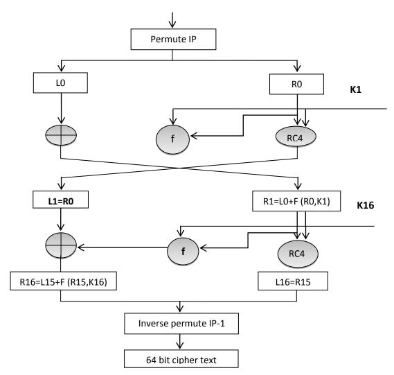
Figure 2: Flowchart to Add RC4 for DES steps.
