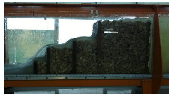
Fig. 2. Caption of Stepped-shape, Rockfill Weir F with Gravel Sample G
