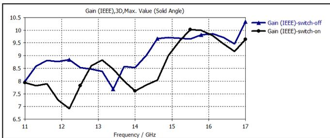
Fig. 4. The gain variation with the frequency of the proposed reconfigurable antenna
