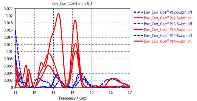
Fig. 6. The simulated envelope correlation coefficients (ECC) of the 4-elements multiband MIMO antenna
