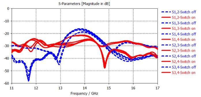
Fig. 5. The simulated isolation of the 4-elements multiband MIMO antenna
