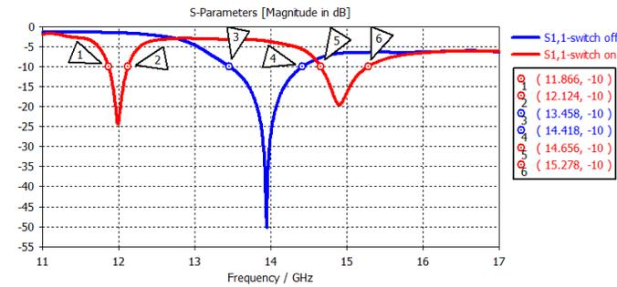
Fig. 3. The simulated (S11) parameter versus frequency of the 4-elements MIMO antenna
