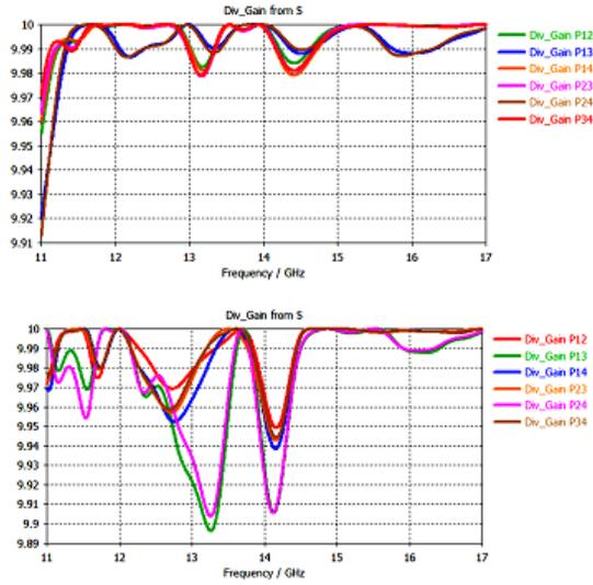
Fig. 7. The simulated diversity gain of the 4-elements multiband MIMO antenna for (a) switch off, (b) switch on.
