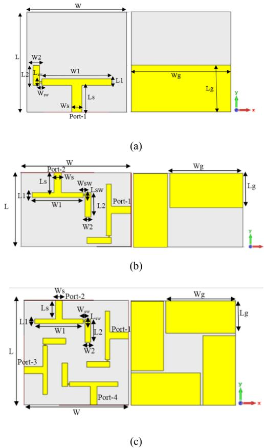
Fig. 1. The proposed multiband MIMO reconfigurable antenna. (a) Single element, (b) 2-elements, (c) 4-elements.
