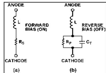
Fig. 2. PIN diode modeling under (a) forward (b) reversed biased condition
