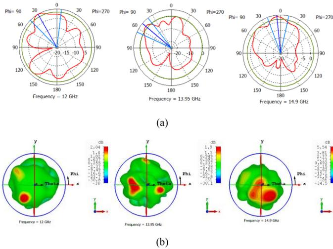
Fig. 7. The radiation pattern of the proposed reconfigurable MIMO antenna for (a) 2D radiation pattern, (b) 3D radiation pattern.
