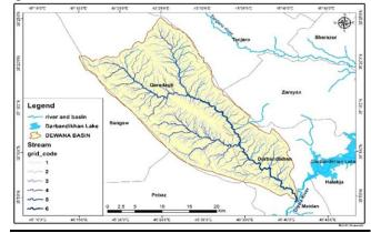
Figure 3: Dewana drainage basin network and sub-basins (Stream from digitizing 1:50000 scale topographic map)
