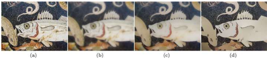
Fig. 1 A comparison on using different global optimization-based edge-preserving filters in texture smoothing. a Input image. b TV [29] ( \lambda = 0.4 ) c WLS [10] ( \lambda = 2, \alpha = 3 ) d L_0 -smoothing [37] ( \lambda = 0.1, \kappa = 2 )
