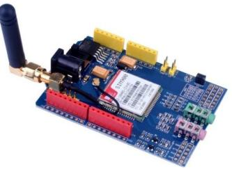
Fig 2 : SIM 900 GSM Shield (Zatin et.al., 2012).
