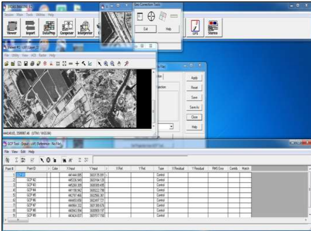
FIGURE 1. Geometric correction of the satellite image using points GCP through ERDAS LPS Imagine.
