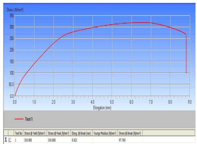
Figure 10. Tensile test diagram for specimen after quenched in (0.1) nano solution the maximum tensile strength value is ( 318.8\text{N/mm}^2 ), as well as the value of hardness Rockwell number is (78.33kgf)
