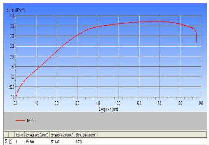
Figure 11. Tensile test diagram for specimen after quenched in (0.2) nano solution the maximum tensile strength value is ( 364.8\text{N/mm}^2 ), as well as the value of hardness Rockwell number is (83.1kgf)
