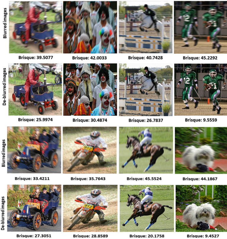
Fig. 17. Deblur images according to the proposed algorithm using Richardson–Lucy Filter
