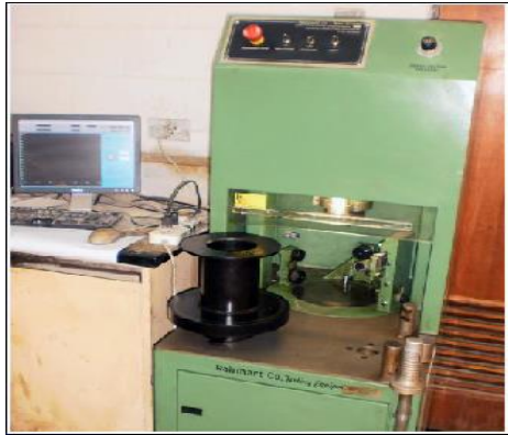
Fig. 5: Gyratory compactor of asphalt concrete
