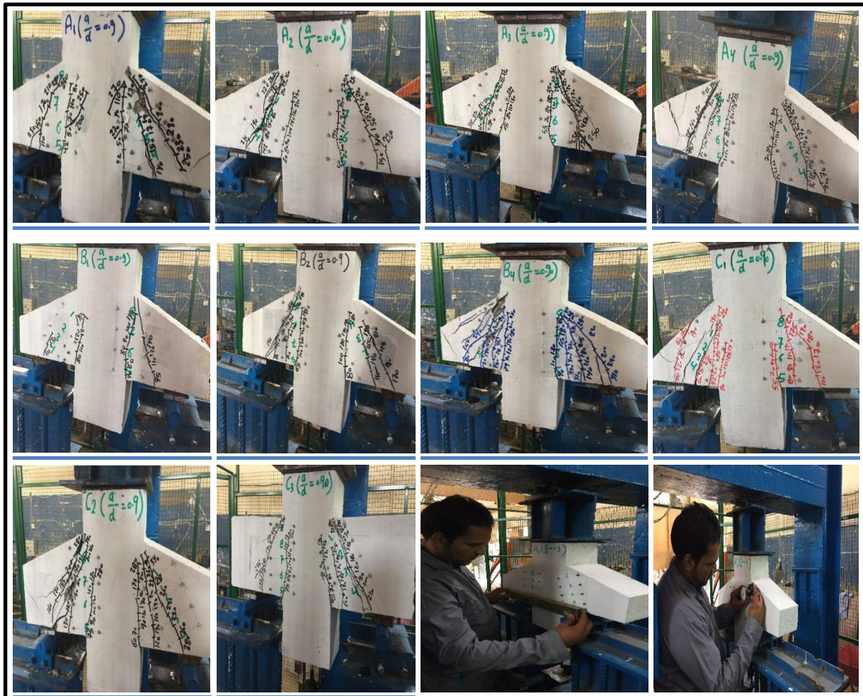
Fig. 10. The Crack Patterns of SCC Corbels under Vertical Loading After Testing.
