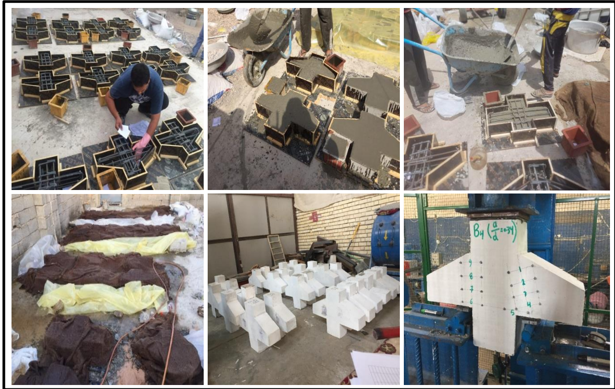
Fig. 3. Casting and Curing Methods of the Reinforced Concrete Corbels Specimens.
