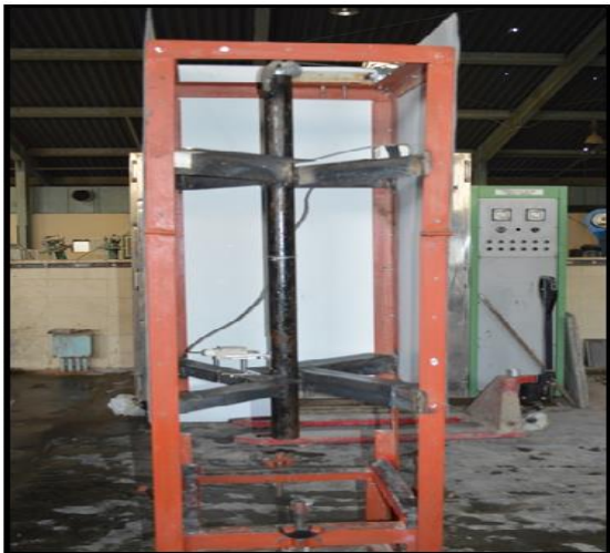
c) Impact Test instrument.
