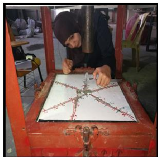
b) Crack width measuring by Vernier Caliper
