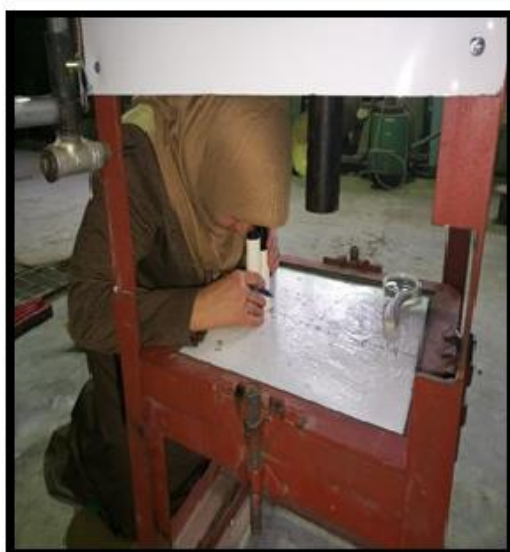
a) Crack width measuring by Portable Microscope.
