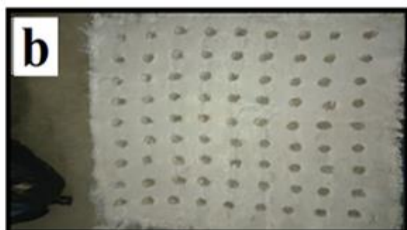
Plates (1): 3D textile glass fiber made in china; a) Zoom view. b) Holes made in 3D glass fiber.
