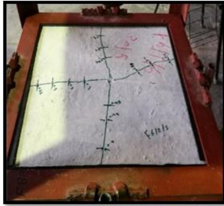
a) Initial Crack of Fixed Support.
