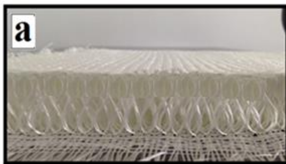
Plates (1): 3D textile glass fiber made in china; a) Zoom view. b) Holes made in 3D glass fiber.
