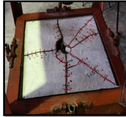
b) Final Crack of Fixed Support.
