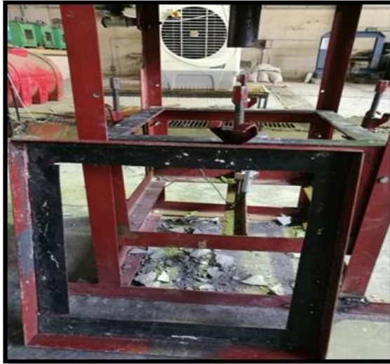
a) Frame of fixed impact test
