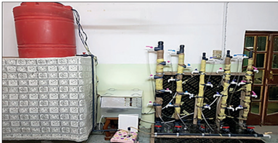
Figure 1. Electromagnetic treatment unit
